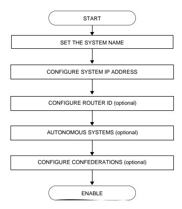
Figure 9: IP Router Configuration Flow
